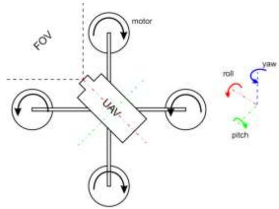
**Fig. 3.** A quadcopter UAV
