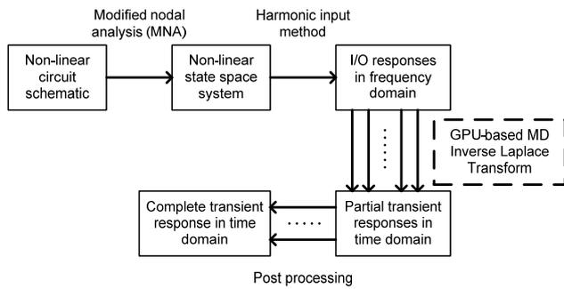
Fig. 1. Overview of an AMS circuit simulation flow.
