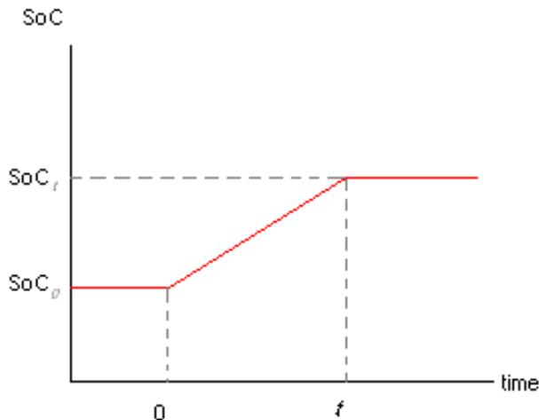
Fig. 1. Estimating SoC by using Coulomb Counting
