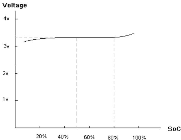
**Fig. 3.** The relationship between Voltage and SoC in Li-ion battery
