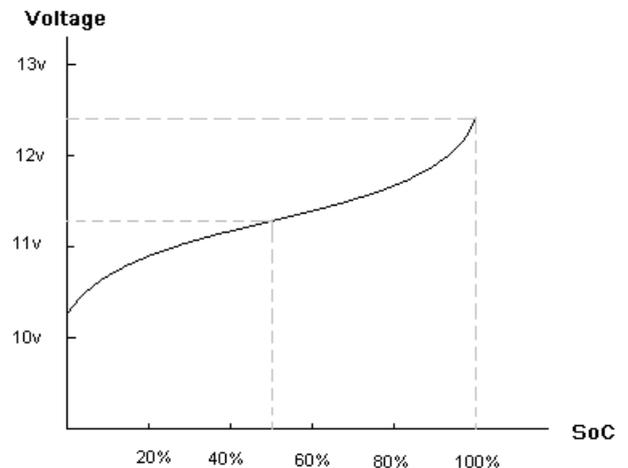
Fig. 2. The relationship between Voltage and SoC in Lead Acid battery
